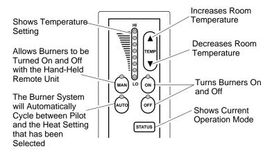
Figure 60 - Hand-Held Thermostat Remote Control Unit Selections (GHRCT Only)
